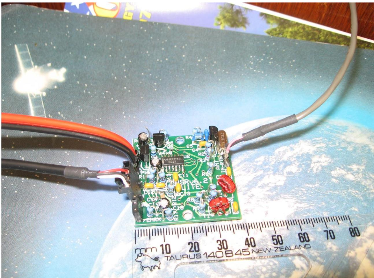
On reading about the SoftRock kits I reasoned that if I could set the device to work at the centre of the 9MHz 1<sup>st</sup> IF in my FT-301 receiver, I would be able to tune to any frequency and still get the advantages of the SDR software. This would effectively add IF DSP filtering, band scope and demodulation to the old receiver. These are features usually only found in the latest top of the range transceivers.
